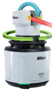
Range to the object is determined through heterodyne interferometry of the laser, meaning high accuracy even with extremely small surface reflection. Coupled with a precise angular position of the mirror, absolute and accurate 3D measurements on almost any surface are possible.
